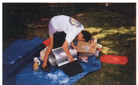
Ken Mizoi adds a smooth fillet to the welded fin can.
