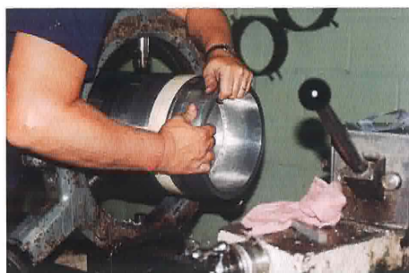
Test fit of the forward closure.
