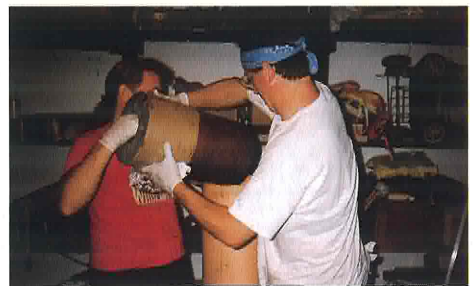
Paul and Jim case-bond the propellant grains into phenolic liners. (Rosson)
