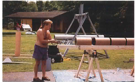
Paul roughs up the core with a pipe brush.
